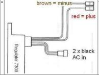
The new regulator/rectifier has 4 wires
