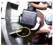
Before you fasten the base plate screws (3 screws M4x12 provided) fully, turn the plate in such a way that the small red marking on its circumference aligns with the stabilisation fin in the casing as shown here.
