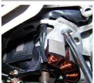
Push the base into the engine recess. Push and pull from the other end the cable so that the stator comes to sit on its base.
