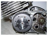
Once ignition position is found, take the rotor carefully off again without changing the crank's position and reset it onto the crank in such a way that the marking on the rotor aligns with the fin of the casing.
