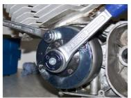
Use of our fastening tool helps, both for setting the rotor and for pulling it again.
