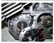
Disconnect the 3 screws holding the stator coil on its base and lift the coil a little, but not fully from the plate.
