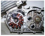
Refasten the coil again with the 3 screws M4x25.
