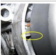
Have a look at the new rotor. You will find on its circumference a small pressed in line. That is an ignition marking too. It is durable, but not well visible, so better highlighten it with some marker pen, preferably on top of the flywheel.
